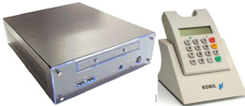
Figure 9: PIN-pad-controlled strongSwan security gateway
